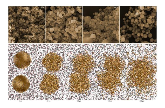
Successive phases of agglomeration of nanoparticles of copper and its oxides, occurring in the first 200 picoseconds of laser melting: top in microscopic images (mag. 50000x), bottom in computer simulation. Credit: IFJ PAN
