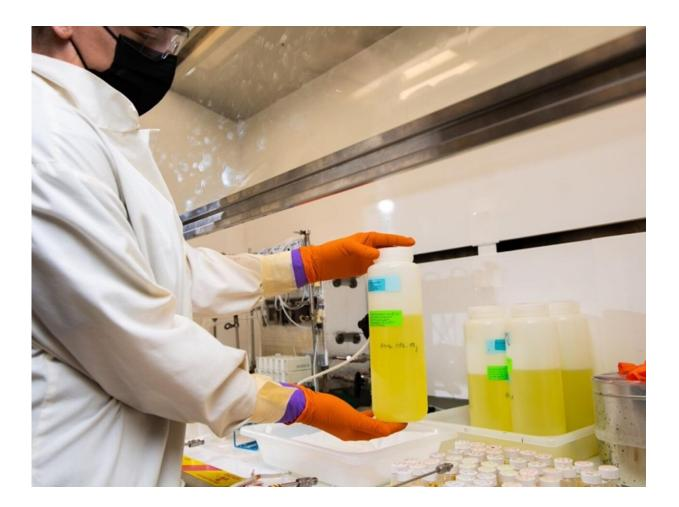
Safe and effective ways to process the Hanford Site's radioactive tank waste, especially to remove cesium as an important pre-treatment step, is researched and developed in the Radiochemical Processing Laboratory at Pacific Northwest National Laboratory. These bottles contain tank waste after the cesium has been removed. Credit: Andrea Starr | Pacific Northwest National Laboratory
