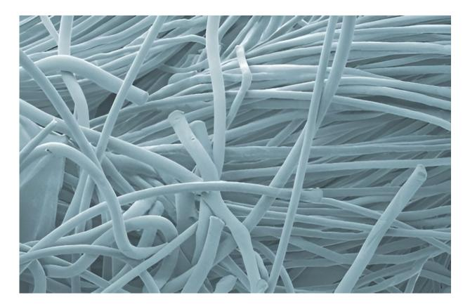
Cellulose-based dressing under a scanning electron microscope. Credit: Empa
