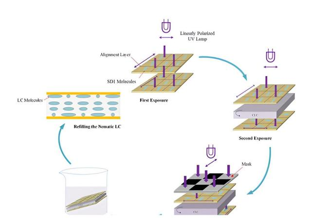
(a) The process for fabricating LC phase modulator with the MMOT structure.(b) The schematic of LC phase modulator with MMOT structure. Credit: by Mingyuan Tang, Kai Huang, Yumeng Zhang and Jiangang Lu
