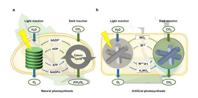
Schematic illustration of the decoupled light and dark reactions in the process of solar-driven  $CO_2$  reduction. Credit: Shi, et al.
