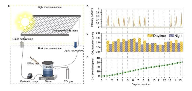
Demonstration of solar-driven CO<sub>2</sub> utilization application. Credit: Shi, et al.
