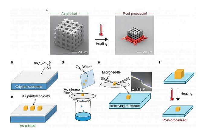
Concept and schematic of the pick and place process for uniform shrinking of 3D printed micro-nano structures. Credit: SUTD, from *Nature Communications* (2023). DOI: 10.1038/s41467-023-41535-9
