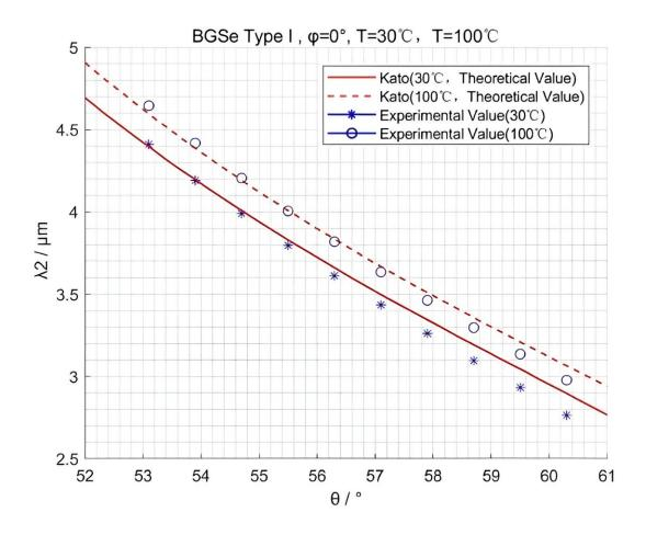
Relationship between output wavelength and angle and temperature. Credit: *Frontiers of Optoelectronics* (2023). DOI: 10.1007/s12200-023-00077-0
