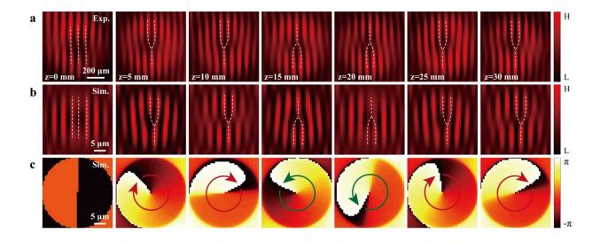
The Rabi oscillation is manifested partially by the separated orbital-angularmomentum oscillation along with the coupling length. a, b, The interferograms recorded at different coupling lengths: a, experiments; b, simulations. c, Simulated phase distributions of light fields at the corresponding coupling lengths. Credit: Guohua Liu, Xiliang Zhang, Xin Zhang, Yanwen Hu, Zhen Li, Zhenqiang Chen, and Shenhe Fu
