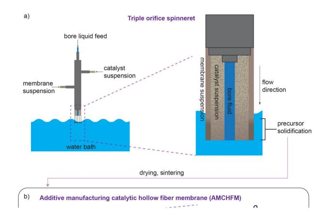
The membrane reactor manufacturing method. Membrane and catalyst layer suspensions are extruded through a triple-orifice spinneret. When the membrane precursor touches water, it forms asymmetric, hollow fibers with a porous, inner catalyst layer. b) The synthesis approach allows for the tuning of the catalyst and membrane layers of the reactor so that reactions between ethylene products and oxygen are minimized. Credit: Linic Lab, University of Michigan
