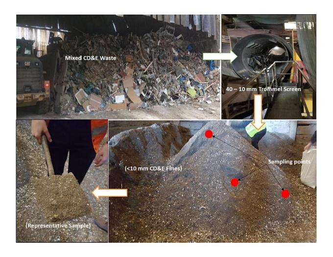
Generation and sampling of trommel fines from CD&E Waste. Credit: *Construction and Building Materials* (2023). DOI: 10.1016/j.conbuildmat.2023.130579
