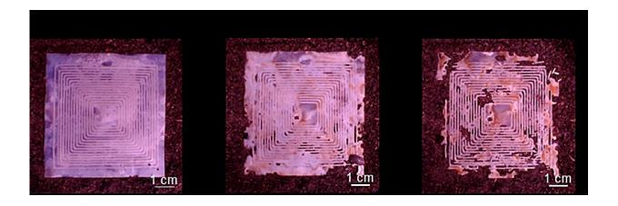
The developed sensor is mostly decomposed by microorganisms in the soil, and the residual components are also environmentally friendly. Credit: *Advanced Sustainable Systems* (2023). DOI: 10.1002/adsu.202300314, CC BY
