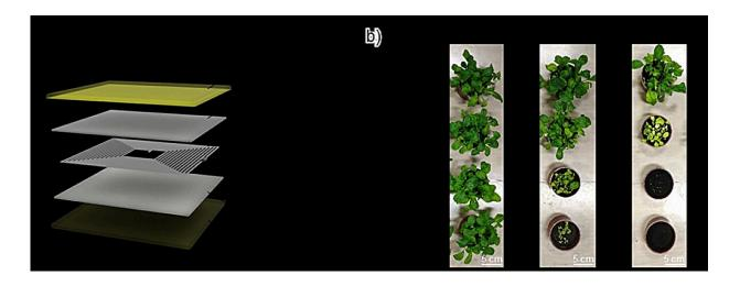
(a) Components and configuration of the degradable soil moisture sensor. (b) Sn used as a conductive material is unlikely to cause plant damage even if it remains in the soil unlike silver (Ag) and copper (Cu). Credit: *Advanced Sustainable Systems* (2023). DOI: 10.1002/adsu.202300314, CC BY
