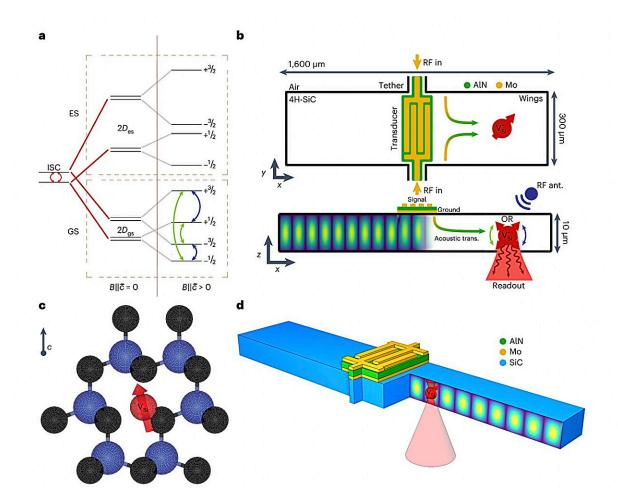
Defect and device structure. a, Electronic structure of V– Si with magnetically allowed and magnetically forbidden but acoustically allowed transitions labeled in blue and green, respectively. Spin polarization is created through ground-state (GS) transduction and then readout by the fluorescence difference between spin
