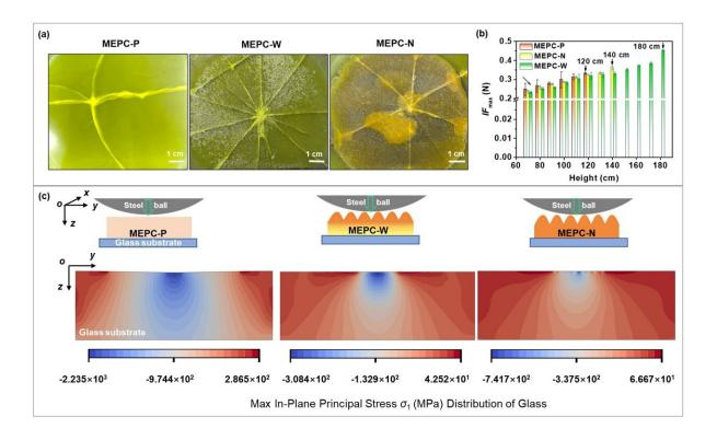
(a) The digital images of the glass substrates coated with different surface coating after crumbling impacted by falling ball. (b) The maximum impact force  $(IF_{\rm max})$  -height curves of pure glass substrate coated with different surface coating. (c) Simulation of anti-impact properties of different surface coating for glass substrates. Credit: Science China Press
