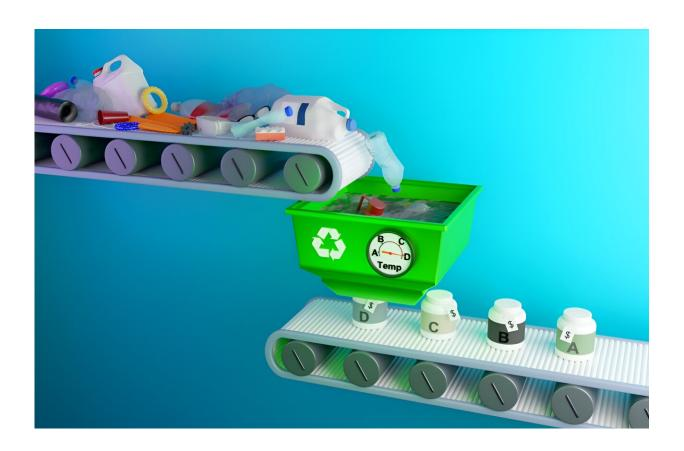
ORNL's organocatalyst deconstructs mixed plastics at different temperatures, which facilitates recovering their individual monomers separately, in reusable form. Credit: Jill Hemman/ORNL, U.S. Dept. of Energy
