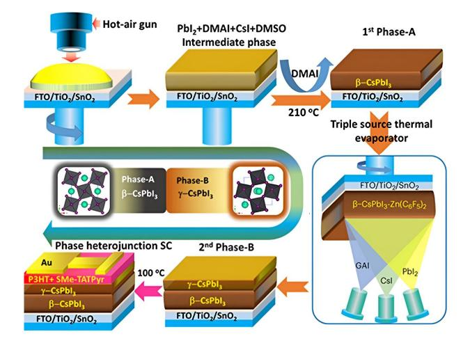
An illustration of a new two-step technique to create stable and efficient next generation solar cells. Credit: Nelson Dzade
