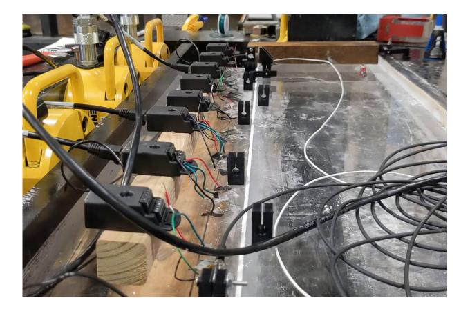
Close-up of the UT Austin lab-fault. The yellow hydraulic presses simulate tectonic pressure while sensors listen for miniature tremors. Chas Bolton, a researcher at UT Austin, is using the device to investigate early-warning tremors. Credit: University of Texas Institute for Geophysics
