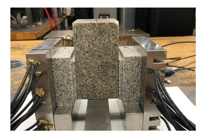
A lab-made fault at Penn State that was used to detect earthquake foreshock patterns in research led by the UT Jackson School of Geosciences. The device squeezes rock blocks in a vice while sensors listen for miniature tremors. Credit: Chas Bolton
