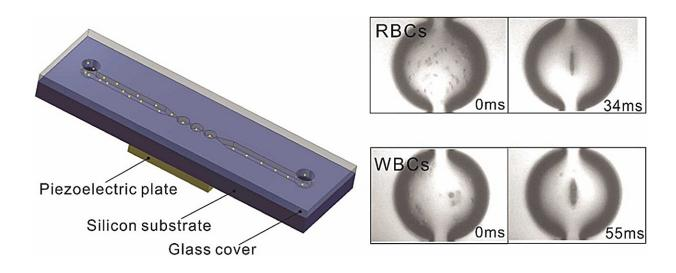
Schematic diagram of the chip design and its trapping performance on red blood cells and white blood cells. The cells aggregate to the center of the circular cavity within 60 ms. Credit: SIBET
