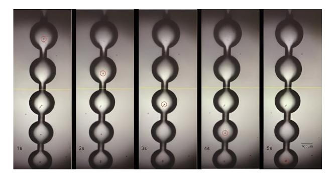
Single particle with diameter of 10 µm queuing up on the cavity array was delivered step by step to the detection spot, which can be applied to high throughput Reman spectra acquisition. Credit: SIBET
