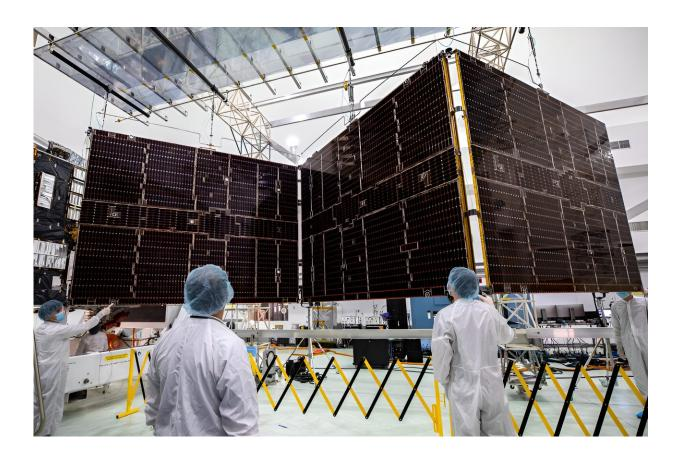
NASA's Psyche mission, a project with deep roots at MIT, is setting course for a metallic space rock that could be the remnant of a planetary core like our own. In this photo, technicians begin to retract one of the two solar arrays attached to NASA's Psyche spacecraft. Credit: NASA/Kim Shiflett
