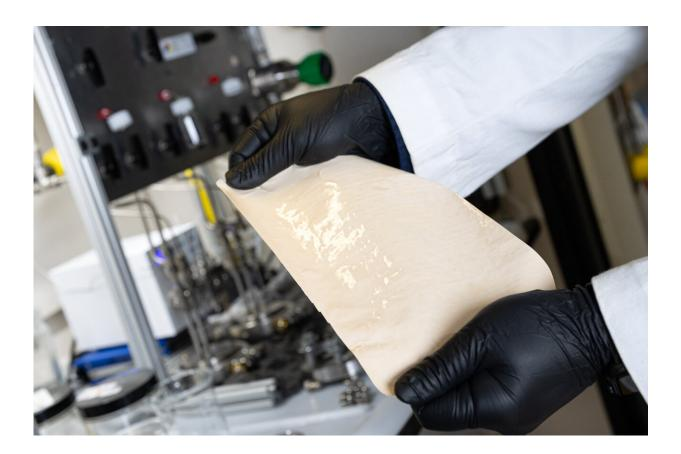
A sample of a DUCKY polymer membrane researchers created to perform the initial separation of crude oils using significantly less energy. Credit: Candler Hobbs, Georgia Institute of Technology
