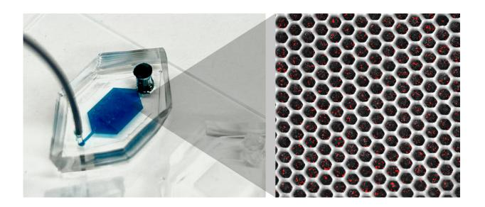
Microwell device with a solution in the reservoir (left) and a visualization of beads capturing extracellular vesicle contents (right). Credit: David E. Reynolds
