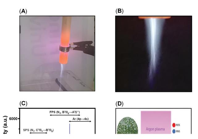
Overview of argon atmospheric plasma jet (Ar-APJ) system. A) Photograph showing the setup argon atmospheric plasma treatment (Ar-APJ) used to transform S. maxima biomass into a robust ultrathin coating. B) Photograph showing the argon atmospheric plasma jet (Ar-APJ). C) OES spectra of Ar-APJ at the argon flow rate of 10 LPM and voltage at 10 kV. D) Illustration of how Ar-APJ can turn S. maxima into a contiguous ultrathin coating. Credit: *Small* (2023). DOI: 10.1002/smll.202305469
