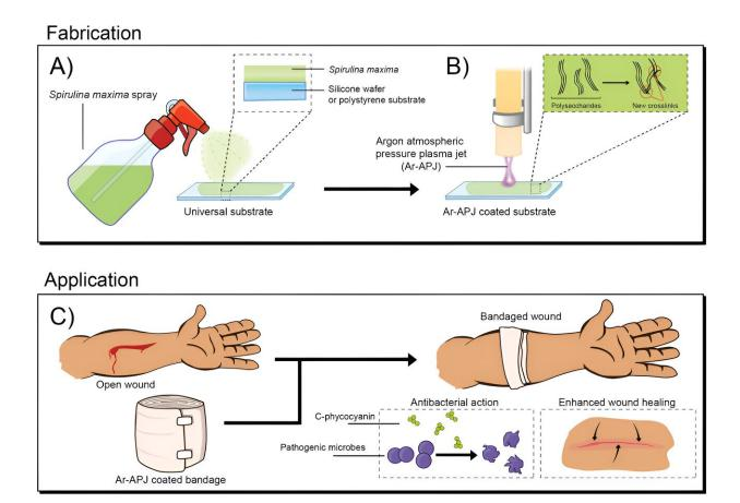
A schematic depicting the one-step argon atmospheric pressure plasma jet (Ar-APJ) process to transform S. maxima biomass into an ultrathin bioactive coating. A) S. maxima is sprayed onto a universal substrate. B) Ar-APJ process transforms the S. maxima biomass into a durable, bioactive, ultrathin coating. C) Antibacterial wound dressings as a proposed application for the Ar-APJ technology. Credit: *Small* (2023). DOI: 10.1002/smll.202305469
