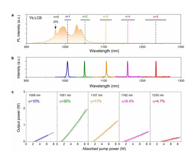
a, Fluorescence spectrum of Y-cut Yb:LCB at room temperature. b, Laser spectrum with different phonon number  $n = 1 \sim 5$ . c, Laser output power versus the absorbed pump power for various phonon numbers. Credit: Yanling Cheng, Fei Liang, Dazhi Lu, Jingcheng Feng, Guochun Zhang, Haohai Yu, Huaijin Zhang, and Yicheng Wu
