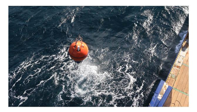
An acoustic current meter, built into a mooring buoy being prepared for deployment in the Atlantic. The ocean current is measured with these instruments. Credit: MARUM – Center for Marine Environmental Sciences, University of Bremen, D. Kieke
