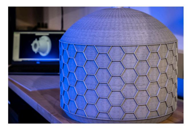
Seen here at the Marshall Space Flight Center in Huntsville, Alabama, and developed with the same 6061-RAM2 aluminum material used under the RAMFIRE project, is a vacuum jacket manufacturing demonstrator tank. The component, made for cryogenic fluid application, is designed with a series of integral cooling channels that have a wall thickness of about 0.06 inches. Credit: NASA
