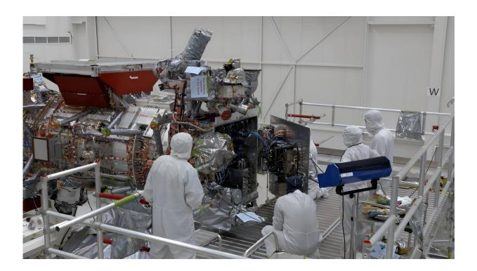
Engineers and technicians are seen closing the vault of NASA's Europa Clipper in the main clean room of the Spacecraft Assembly Facility at JPL on Oct. 7. The vault will protect the electronics of the spacecraft as it orbits Jupiter. Credit: NASA/JPL-Caltech
