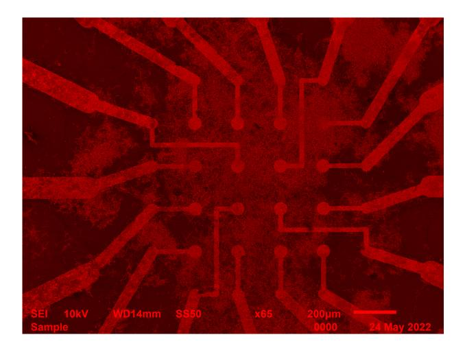
Electron microscope image of electrode interaction with the nanowire neural network. Credit: The University of Sydney
