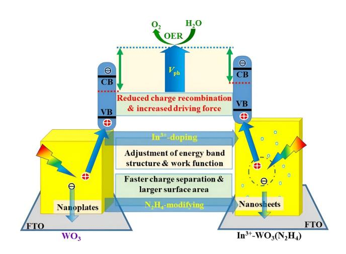
Hydrazine hydrate in the hydrothermal solution promotes the formation of layered WO<sub>3</sub> film stacked by (020) facet-exposed nanosheets, while  $In^{3+}$ -doping optimize the electronic band structure of WO<sub>3</sub> to enhance the OER driving force. Credit: Science China Press
