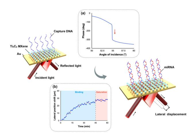
Schematic diagram of miRNA detection scheme based on phase-induced lateral displacement measurement. Inserted figure (a) Sensing mechanism based on a sharp phase change. (b) Sensing signal upon miRNA injection. Credit: *Nanophotonics* (2023). DOI: 10.1515/nanoph-2023-0432
