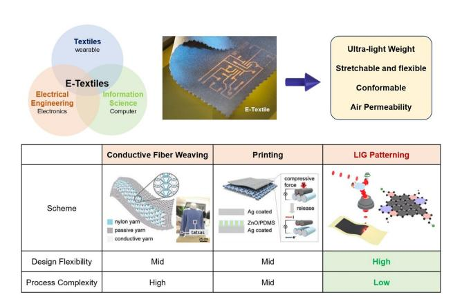
(Above) Introduction on e-textiles and (below) comparison of methods for manufacturing e-textiles. Credit: Korea Institute of Machinery and Materials (KIMM)
