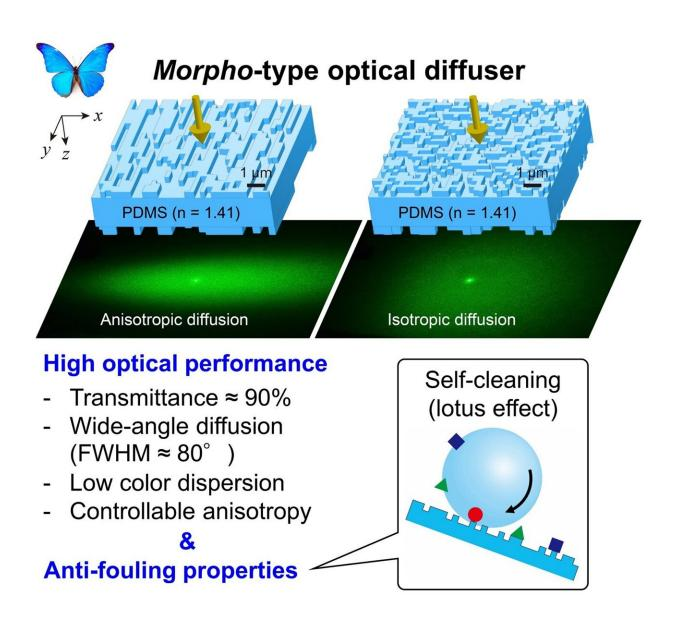
Design and diffused light for the anisotropic (left) and isotropic (right) Morphotype diffusers. It has high optical functionalities and anti-fouling properties,
