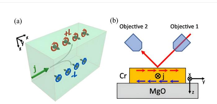
a) Schematics of the orbital Hall effect. The charge current *j* generates a transverse orbital current, leading to orbital accumulation on the sample's surfaces. (b) Measurement setup utilizing the longitudinal MOKE to detect the inplane orbital accumulation. Credit: *Physical Review Letters* (2023). DOI: 10.1103/PhysRevLett.131.156702
