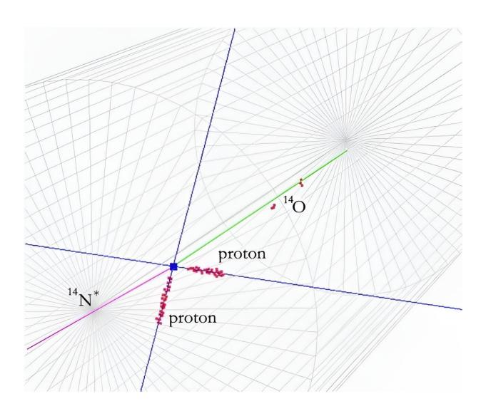
Visualization of a (deuteron, helium-2) reaction on an oxygen-14 nucleus. The Active-Target Time Projection Chamber observes tracks from two protons
