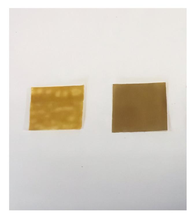
Membrane films containing MOFs, like those shown here, that produce nitric oxide could provide antibacterial properties in medical devices. Credit: Adapted from ACS *Applied Materials & Interfaces* 2023, DOI: 10.1021/acsami.3c11283
