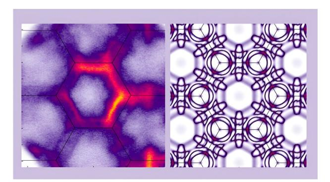
Electronic structure measurements and calculations of  $NiTa_4Se_8$ . Credit: Berkeley Lab
