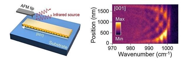
The tip of an atomic force microscope (AFM) focuses infrared (IR) light from an X-ray beamline onto a tiny spot, enabling researchers to detect the lattice vibrations of an ultrathin, ribbon-like nanocrystal (yellow). Credit: Lawrence Berkeley National Laboratory and Stanford University
