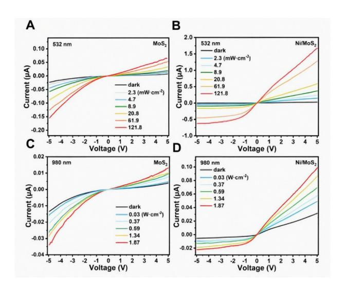
The I-V curves of MoS2 device (A) under 532 nm illumination and (B) 980 nm illumination; the I-V curves of Ni/MoS2 device (C) under 532 nm illumination
