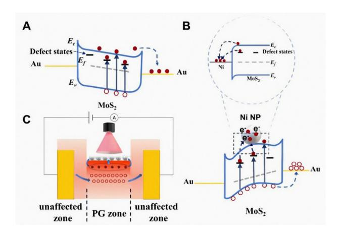
(A) Energy band diagram of MoS2 device under negative voltage, (B) energy band diagram of Ni/MoS2 device under positive voltage and zoom-in energy band structure of Ni NP and MoS2; (C) schematic illustration of the transport
