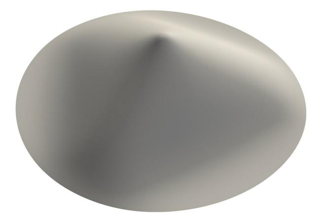
A squashed cone buckles near its boundary, forming a transitory triangular pyramid. Credit: Duffy et al.
