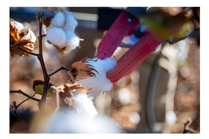
The newly developed "end-effector," a two-fingered robotic arm developed as part of an autonomous agriculture focus at Mississippi State, harvests cotton. Credit: David Ammon
