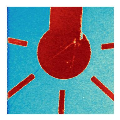
Photoluminescence image showing NV centers near a network of five artificial synapses in a  $VO_2$  film. A central electrode resembling a dendrite is connected to power sources, while five labeled electrodes A to E act like presynaptic terminals. Credit: Ce Feng, DOI: 10.1126/sciadv.adg9376
