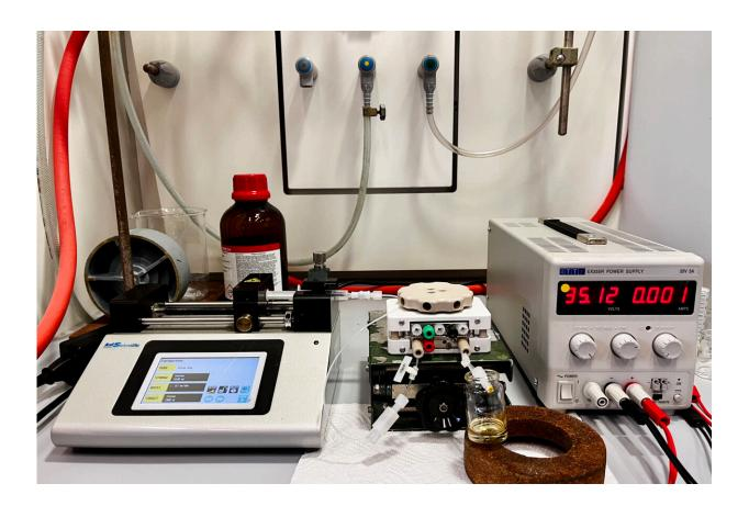
The device takes the form of a small box in which the reaction medium circulates between two electrodes producing the electric field. Credit: Stefan Matile
