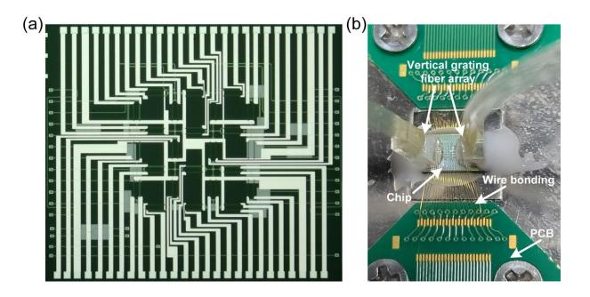
Researchers have created an optical chip that is based on a quadrilateral Mach–Zehnder interferometer network and is easy to reconfigure for various functions. Pictured are a microscope image of the chip (a) and a photo of the packaged chip (b). Credit: Jianji Dong, Huazhong University of Science and Technology
