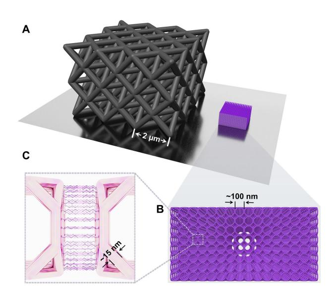
Schematic of 3D-printed and DNA assembled lattices.(A) Schematic showing
