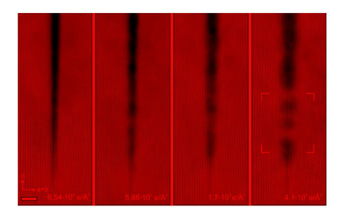
These electron microscope images show how the crack in a crystal of titanium dioxide begins to "heal" with increasing electron doses. Credit: Mkoyan Group, University of Minnesota
