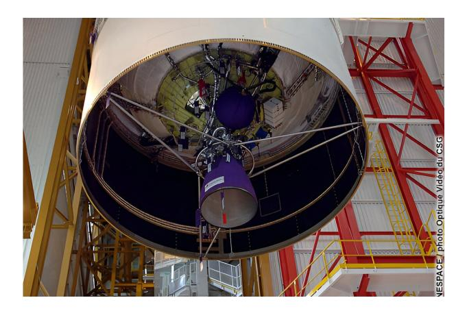
The cryogenic upper stage (Etage Supérieur Cryotechnique de type A—ESC-A) for Ariane 5 ECA flight V172 being hoisted prior to integration on top of the main body of the launcher. The integration was performed in the Launcher Integration Building (Bâtiment d'Intégration Lanceur—BIL) at Europe's Spaceport at Kourou in French Guiana on 19 June 2006. Credit: ESA/CNES/ARIANESPACE-Service Optique CSG
