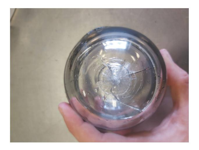
Breaking glass spheres which generates sounds at a level that marine mammals use at great depth, which are then recorded from tens to hundreds of kilometers away. Credit: NIOZ
