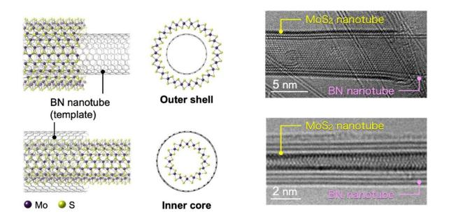
Boron-nitride nanotubes can template the growth of TMD nanotubes both inside and outside the tube. These can be directly observed by transmission electron microscopy (right). Credit: Tokyo Metropolitan University
