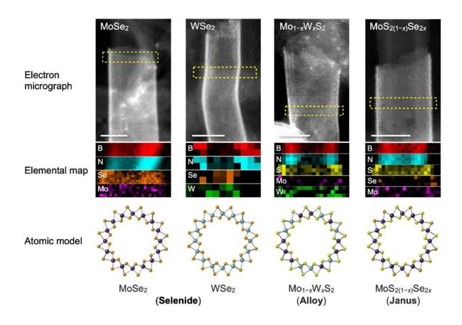
Electron microscopy images of newly realized TMD nanostructures (top), distribution of elements across their cross-section (mid), and their atomic structure (bottom). Credit: Tokyo Metropolitan University
