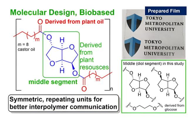
Basic design, structure of present biobased polyesters Basic structure, framework in the present biobased polyesters derived from plant oil and glucose (in this study). The present polymers can be easily decomposed to the monomer units by chemical recycle simply using treating with alcohols (called catalytic transesterification). Credit: JST
