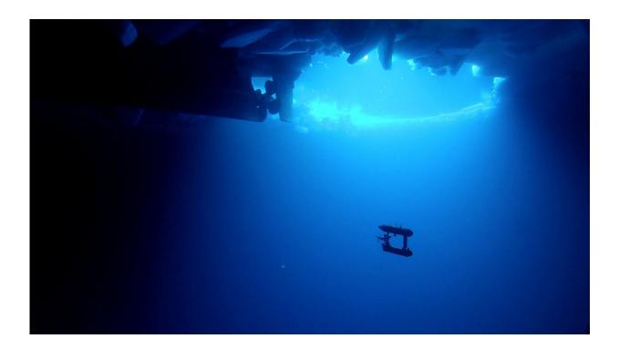
Remote sensing instruments on autonomous underwater vehicles will play a role in the Ross Sea far East Antarctic observing system. Credit: ROV team
