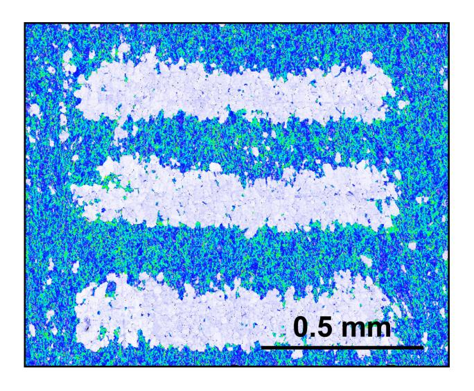
A scanning electron microscope photo of a stainless steel part 3D printed using the new method developed by NTU Singapore and the University of Cambridge. The white regions of the metal part are mechanically weak, while the blue-green regions are strong. Credit: NTU Singapore
