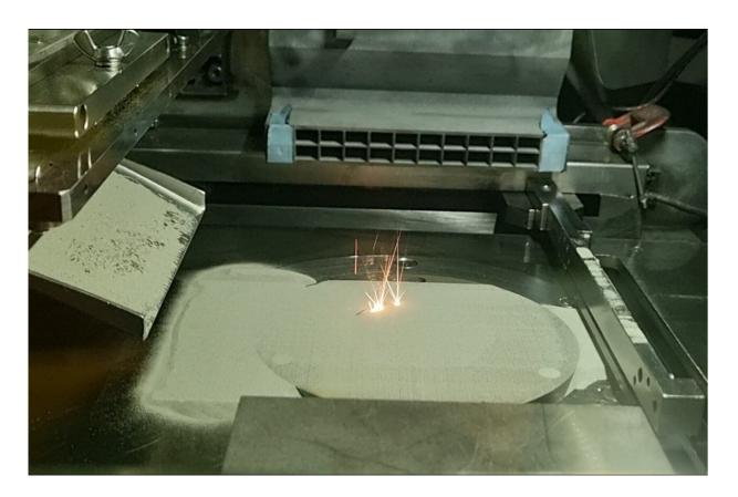
One of the laser powder bed fusion machines used in the experiments by NTU Singapore and the University of Cambridge to 3D-print metals with different properties. Credit: Jude E. Fronda
