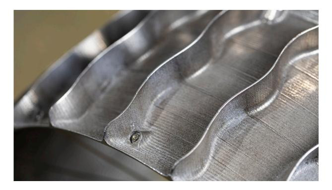
Additive manufacturing allows fine design details, such as wavy tread on a domed shape, to be incorporated into the prototype lunar wheel. Credit: Carlos Jones/ORNL, U.S. Dept. of Energy
